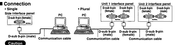
· Purchase an appropriate communication cable to connect a computer to the serial terminal.
