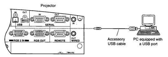
• When your PC is attached to the projector for the first time, the "new hardware wizard" will launch automatically. When USB cable connects for the first time between projector and PC, the following massage appear from PC. The reason that the driver not installed, therfore press "NEXT" button continuously and finally. Press "Finish".
