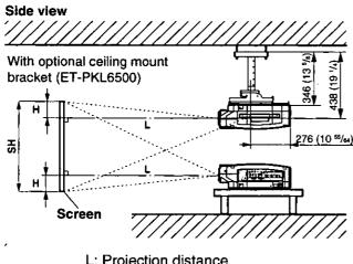
L: Projection distance SH: Image height SW: Image width H: Distance from center of lens to bottom
